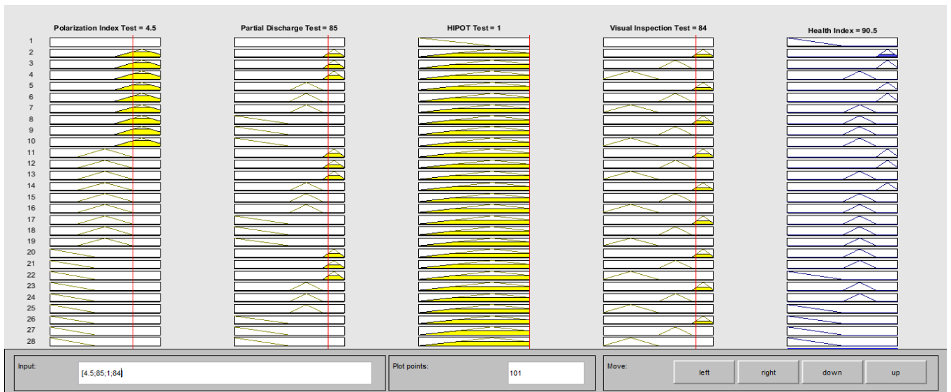
Fig. 15 Fuzzy Inference Diagram for Gen no. 3 and Execution of Rule no. 2.
