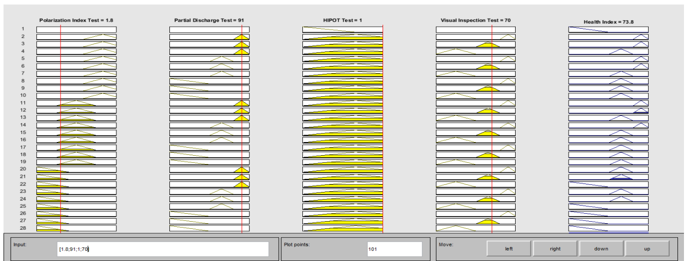
Fig. 14 Fuzzy Inference Diagram for Gen no. 2 and Execution of Rule no. 12 and 21.
